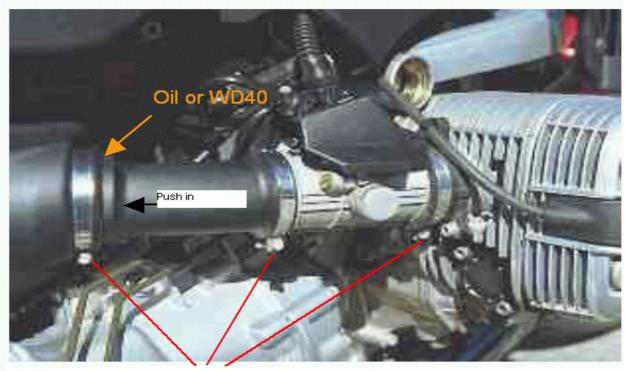
Loosen all three clamps. Push the funnel back into the air filter casing by slithly turning it. If need be, add a little oil or Q20 as indicated in the drawing. Take off the throttle unit. Be carefull not to break the plastic pipe.
